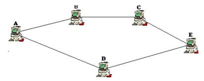
Suppose that computer A wants to send a large message to computer E using B, C, and D as intermediate switches. The network shown provides two paths from A to E. One path goes B and C and the other goes through D. While the network itself is unrealistically simple, the presence of such multiple paths is not unrealistic. Multiple paths are desirable because they provide reliability in the case that a link is damaged.
