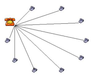
If such a company wanted to interconnect more than two offices, it would have to install wires between every pair of offices. The diagram on the left illustrates the wiring needed from the point of just one office in such a system.
