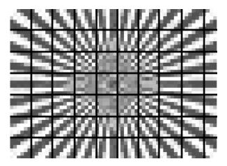
Next, compute the average brightness of the pixels in each cell of this grid and then replace the colors of all the pixels within each cell with the average brightness. Looking through our imaginary grid, the new image will look like:
