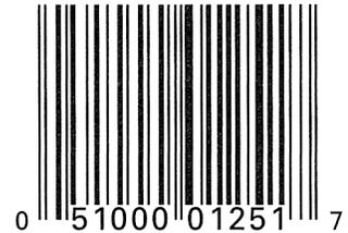
The black and white bars in a UPC are simply an encoding of the twelve decimal digits that appear below them (05100012517 in this case). The bars encode this information using a system designed to be easily read by devices attached to cash registers at super market checkout counters.
